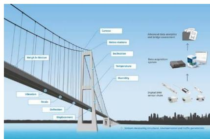
Kistler will present its fully digital structural health monitoring solution for bridges for the first time at Intertraffic 2026 in Amsterdam (hall 1, booth 410, March 10-13). The modular measurement system offers continuous monitoring and structural insights to support proactive maintenance, extend bridge service life, and improve traffic safety.
