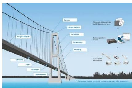
Kistler showcases its fully digital structural health monitoring solution for real-time bridge monitoring for the first time at Intertraffic 2026 in Amsterdam (hall 1, booth 410, March 10-13). The modular measurement system offers real-time insights into structural conditions of bridges to support proactive maintenance, extend bridge service life, and improve traffic safety.
