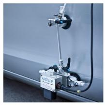
Combining optoelectronic speed sensors with inertial sensors provides precise movement and velocity data for every road segment, enabling context-aware analysis of road pavement quality.
