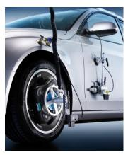
High-dynamic acceleration sensors and laser height sensors mounted on test vehicles capture road surface profiles with exceptional resolution, forming the foundation for accurate road surface quality assessment during construction.
