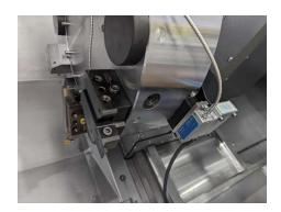
With Kistler's new telemetric measurement system, wireless, wear-free signal transmission is possible for the first time in tool monitoring of rotating structures.
