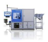
The KVC 821 optical inspection system reliably detects surface and dimensional defects in plastics manufacturing.
