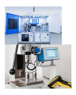
The KVC 821 optical inspection system from Kistler performs automated quality assurance at the end of the production line.
