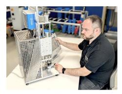
The new NCFQ high-speed joining system from Kistler combines a LinMot linear module with precise piezoelectric measurement technology. It is ideal for demanding joining applications with high dynamics – especially in the medical, electronics, semiconductor, and automotive industries.
