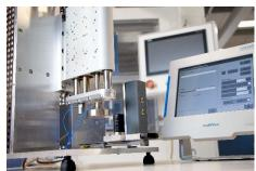
High-speed joining meets precise force measurement: Kistler supplements the proven LinMot linear module with piezoelectric force measurement technology and automatic acceleration compensation.
