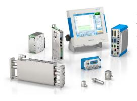
The advanced high-speed joining system with acceleration compensation consists of a joining module with linear motor, servo drive, switching power supply, one force sensor and one acceleration sensor, the corresponding ICAM-B industrial load amplifier, and the maXYmos NC process monitoring system.
