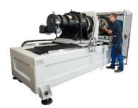
New calibration service: Kistler offers accredited torque calibrations according to ISO 17025 as well as factory and service calibrations in the range from 5,000 to  $100,000~N\cdot m$  – also for third-party products.
