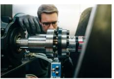
The KiTorq 4552A torque measuring flange system from Kistler can be applied on an electric motor test bench, for example.
