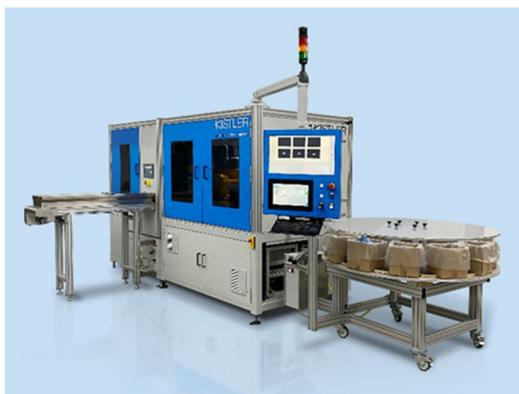
The Automated Vision Inspection system achieves, depending on the configuration, cycle times of two seconds from the moment the test piece is picked up to the OK/NOK decision and the corresponding sorting.
