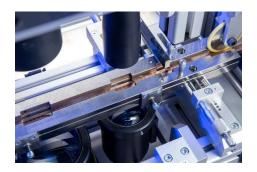
The KiVision image processing software from Kistler can detect deviations from dimensions or contours as well as relevant surface defects. It also offers Al-based anomaly detection.
