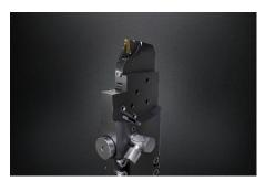
Kistler developed the Piezo Tool System (PTS) in cooperation with HORN in order to continuously monitor cutting tools for microprocessing - see it for yourself at EMO Hannover. | © HORN/Sauermann
