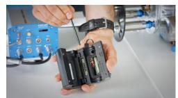
The adapter for the transmitter is tailored to drive shaft for an optimal fit.
