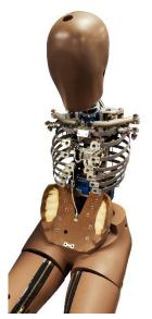
The new THOR 5F ATD features improved biofidelity and easier assembly. The simplified rib structure is shown here.
