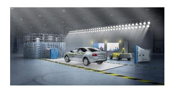
Engineers can simulate realistic test situations using integrated crash test measuring systems supplied by Kistler. Shown here is a typical setup with crash block and crash wall along with a fixed and mobile multibarrier from ERNST.
