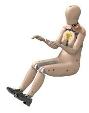
The THOR 5F crash test dummy simulates vehicle occupants that are smaller and lighter than average.
