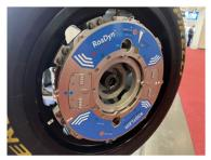
With the new wireless RoaDyn Racing wheel force transducer, Kistler is expanding its leading RoaDyn range of wheel force transducers to include motorsport applications.
