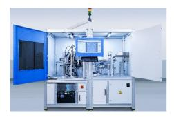
Thanks to artificial intelligence and anomaly detection, the KVC 821 automatic optical testing system can identify the very smallest defects – even those that were previously unknown.
