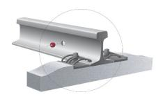
The core of the new Rail WIM solution from Kistler is the improved piezoelectric sensor 9008B (in red) which is installed into the rail tracks in an optimized layout of twelve sensors in six pairs.
