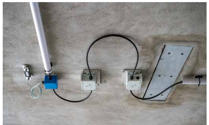
Multi-sensor set-up with acceleration and strain measurements
