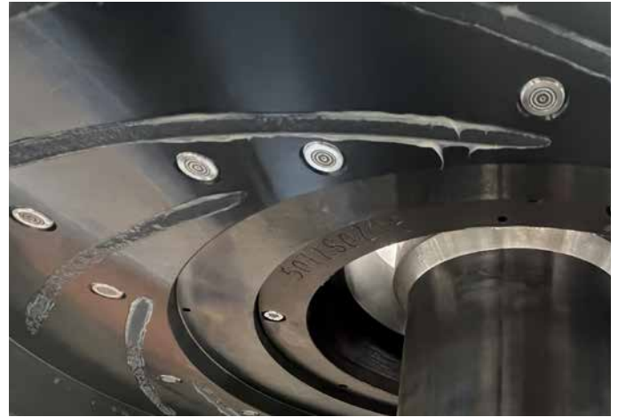
Inside view of a pump component in development, with flush-mounted pressure sensors from Kistler.
