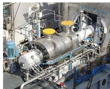
Sulzer HPcp high-pressure centrifugal pumps were developed using measurement technology from Kistler. They set new benchmarks in the industry, for example in water injection for oil production.
