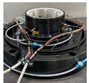
Pump development: outside view of an instrumented component equipped with pressure sensors and cabling.
