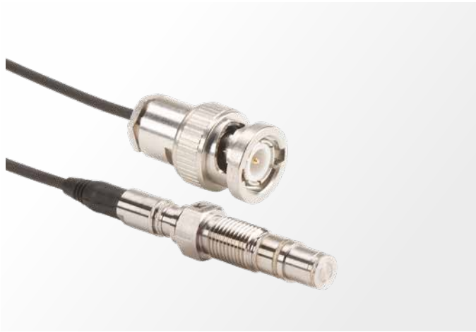
The 603C pressure sensor from Kistler is a compact and robust piezoelectric transducer, available in many different versions including a waterproof (IP68) version for flush mounting in fluid testing.
