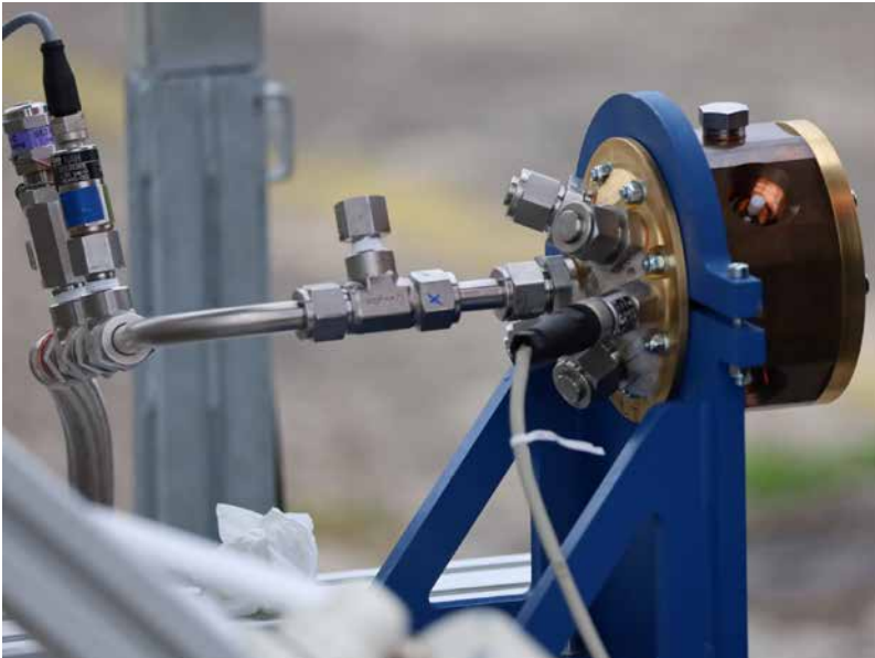
Innovative rocket engine: structure of the rotating detonation rocket engine (RDRE) developed by ARIS Perseus with the annulus (ring-shaped space) and inlets for the fuels.
