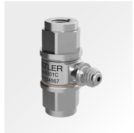
Three 9301C piezoelectric force sensors from Kistler series are installed in the proofload testing machine to measure forces of up to 4 kN over a maximum duration of 99 seconds.
