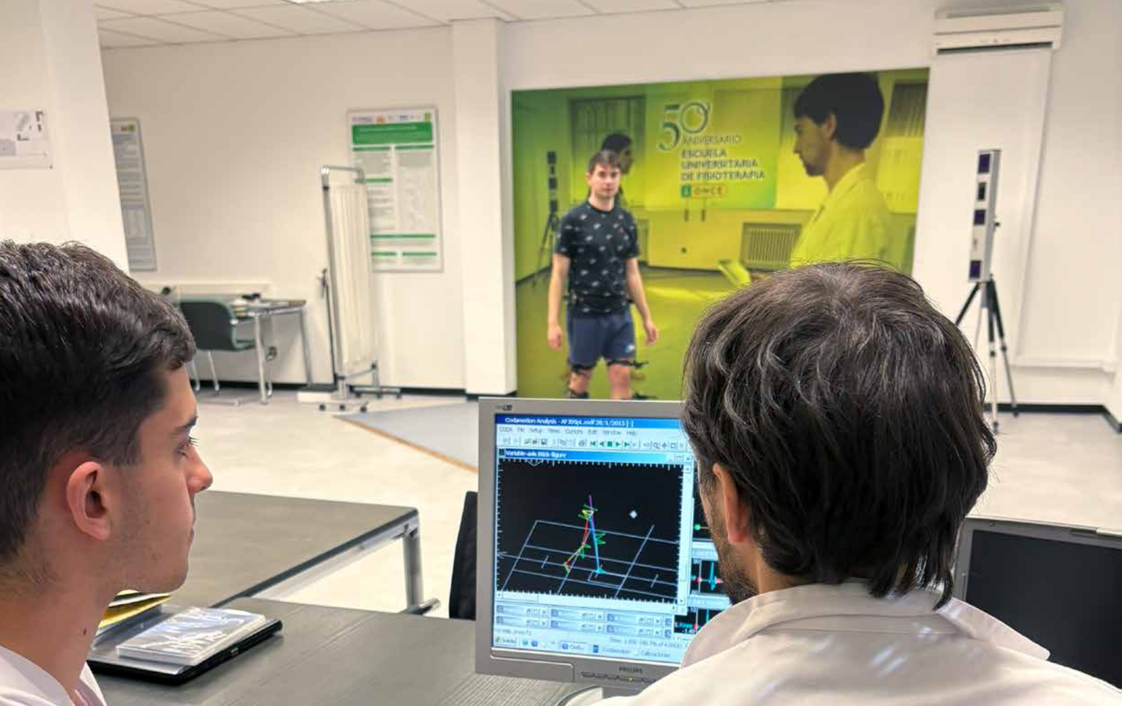
In the gait laboratory at the ONCE University School of Physiotherapy at UAM, instruments such as cameras, body markers and a force plate from Kistler are combined to obtain comprehensive biomechanical data.
