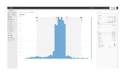
The histogram function supports statistical process control for evaluating production batches in injection molding regarding process capability within the desired intervention limits.
