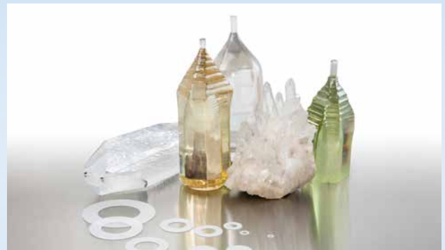
Kistler has developed and grown its own crystal to replace traditional quartz for the most challenging piezo dynamic force measurement applications.
