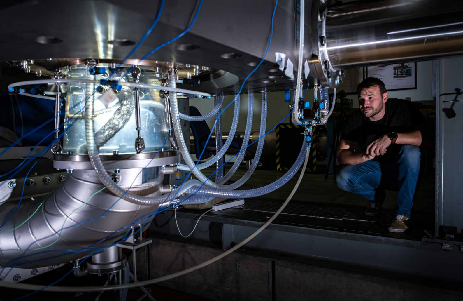
Cavitation is visualized during model acceptance tests on a scaled-down physical model of a pump- turbine, installed on the EPFL turbine test stand (image: PTMH).
