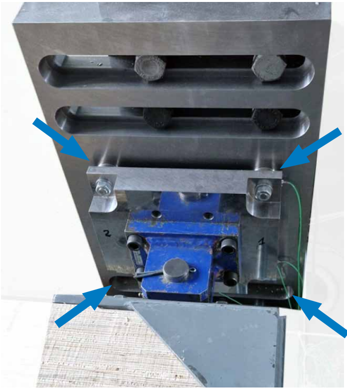
Impact testing: four 9051C piezoelectric force sensors from Kistler are installed in a rectangular layout under a plate at each side of the support system holding the timber beam in position.
