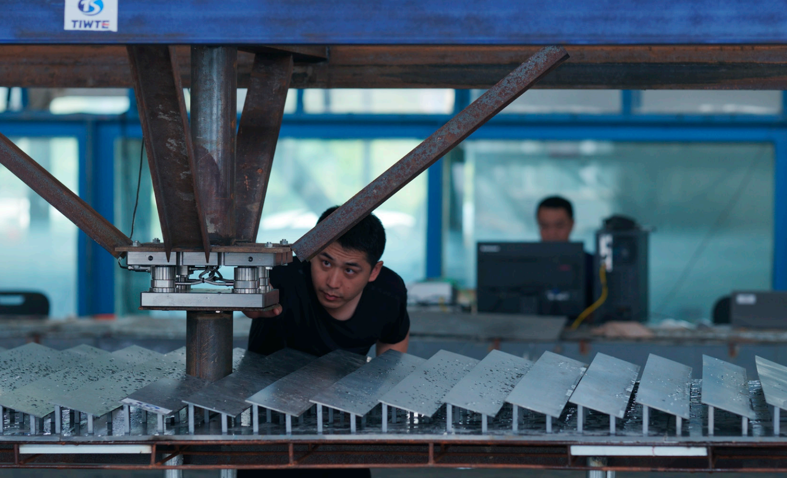
Offshore structures test: Dr. Hu Jielong of TIWTE inspects the installation of Kistler's waterproof dynamometer under the platform for a photovoltaic system installed at sea.
