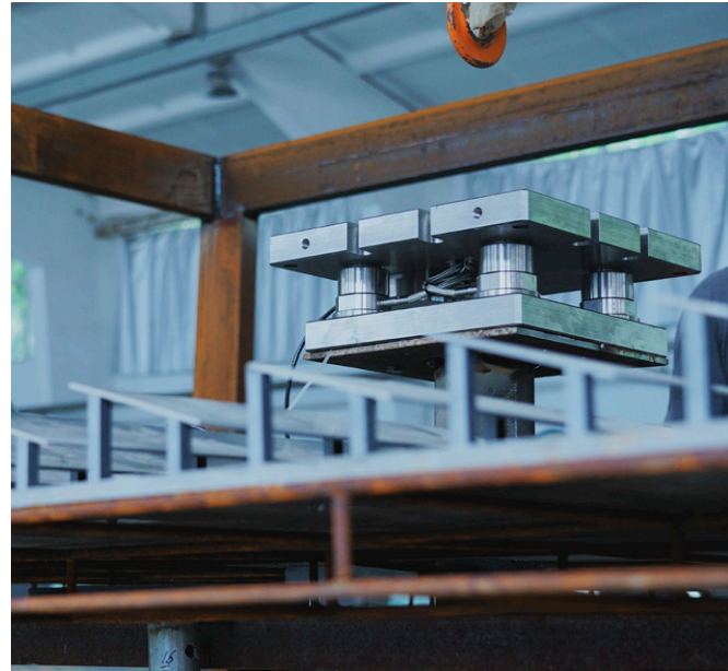
A dynamometer developed by Kistler for hydrodynamic tests provides researchers at TIWTE with precise measurement data – even under extreme conditions.
