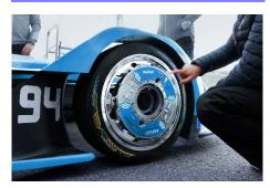
The new RoaDyn Racing wheel force transducer from Kistler plays a key role in developing the latest GT3 vehicles. It has also proven its capabilities in Formula E since 2021 with a pre-series version.
