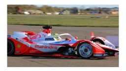
The RoaDyn Racing wheel force transducer is equipped with four highly precise sensors that measure the moments and loads affecting the wheels. It enables motorsport teams to optimize race strategy and tire management, and significantly enhances safety for both drivers and spectators.
