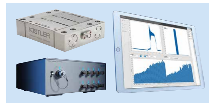
The Kistler measuring chain at Chalmers comprises the 9139AA MiniDyn multicomponent dynamometer (top left), the LabAmp 5167A laboratory charge amplifier (bottom left), and the PTS app software.
