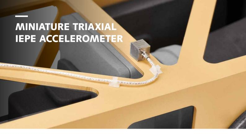
KiVibe Miniature: The perfect fit for vibration measurements on lightweight structures and in tight spaces
