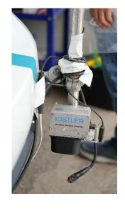
Accurate, real-time speed and slip angle data is key to optimizing tire performance, made possible by the Correvit S-Motion optical sensor's advanced measurement technology from Kistler, which captures vehicle motion without contact to provide accurate data under varying road conditions.
