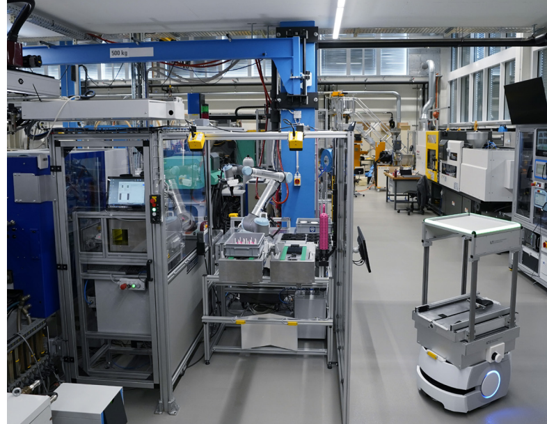
The autonomous vehicles transport the parts to the test cell and then to the storage area for retained samples
