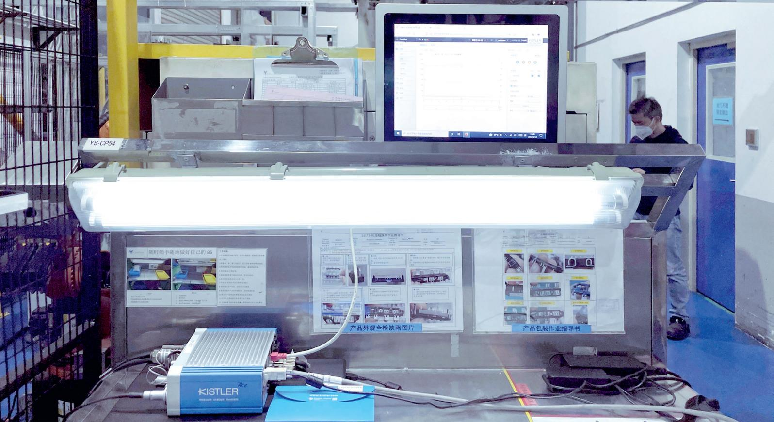
A manufacturing cell at Schneider Electric GSC China: scrap rates were significantly reduced by integrating cavity pressure and temperature sensors, together with the ComoNeo process monitoring system from Kistler.
