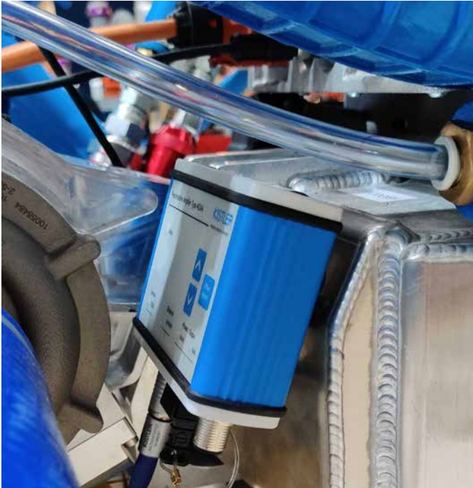
A 4624AK amplifier from Kistler is integrated in the Forze IX motorsports race car from Forze Hydrogen Racing; it transmits signals from different piezoresistive pressure sensors to the hydrogen car's control system.
