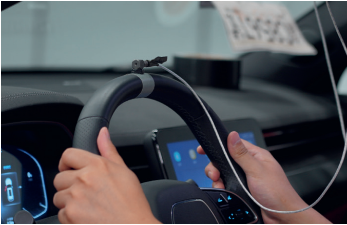
An 8763B accelerometer from Kistler is mounted on a steering wheel for NVH testing at the China Automotive Engineering Research Institute (CAERI) in Chongqing.
