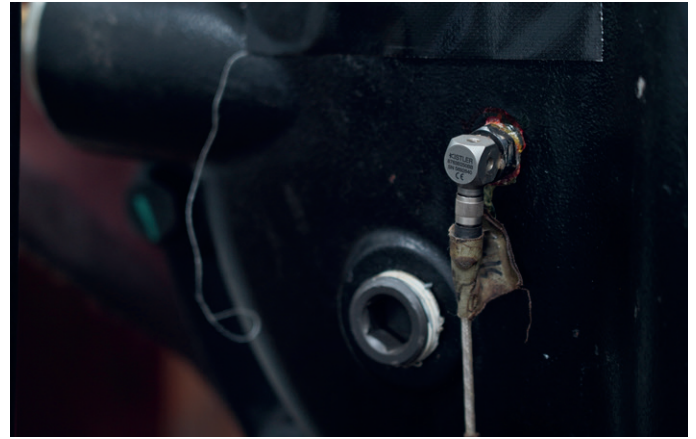
For NVH analyses of powertrains, components and auxiliary systems, the engineers at CAERI rely on force and vibration sensors from Kistler – such as this 8763B ceramic shear miniature IEPE accelerometer.
