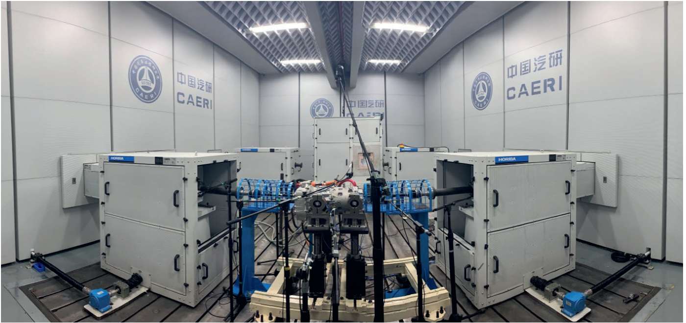
In CAERI's electric powertrain laboratory, Kistler measurement technology plays a key part in advanced NVH testing for new energy powertrains.
