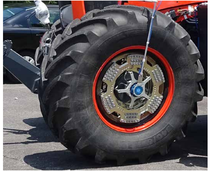
To optimize use of the RoaDyn S6XT wheel force transducer, Kistler provided Kubota with special mechanical adapters for various tractor types and installation conditions.
