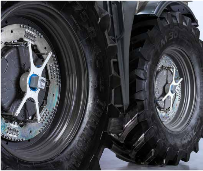
Largest wheel force transducer from Kistler, the RoaDyn S6XT, will be applied for the further development of Kubota tractors, too.
