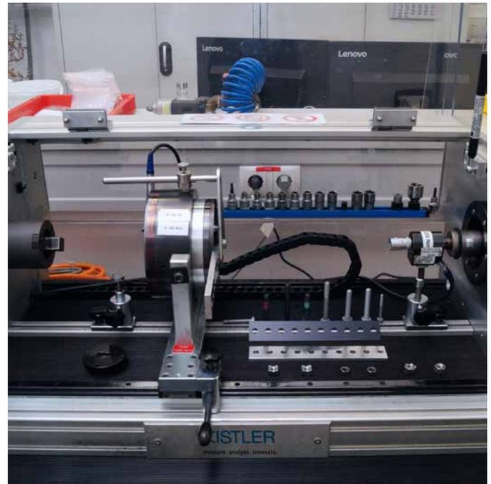
The laboratory test stand for precise determination of friction coefficients: the ANALYSE system from Kistler features a modular structure, and it can be equipped with multiple drives and a vibration test stand.
