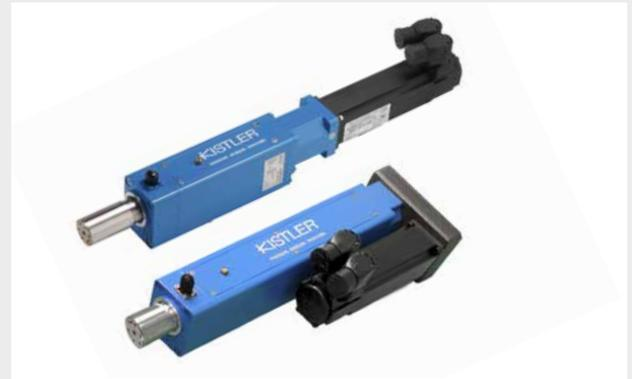
The NCFT joining module from Kistler (Type 2157B) for low compression forces up to 1.5 kN is available in two versions: straight (with a stroke of 100 mm) and a compact angular variant (stroke: 250 mm).
