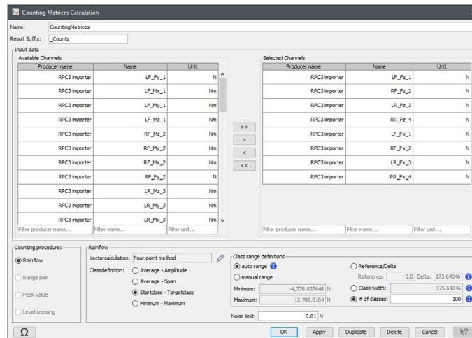
The Rainflow analysis determines a two-dimensional distribution. It is mainly used to analyze life expectancy. The results are output as a matrix.
