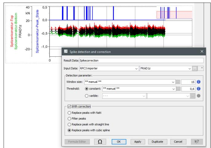
The calculation determines outlier values in a measuring signal and corrects them in a definable mode. Spike detection is easy to configure by defining a range of permitted values.
