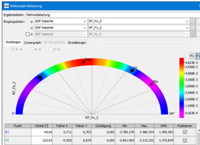
Preparation of single-axial trials in which load signals are vectorially combined in two or three directions and assessed using the damage:
