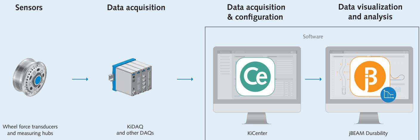
From sensor to software – the complete measuring chain
