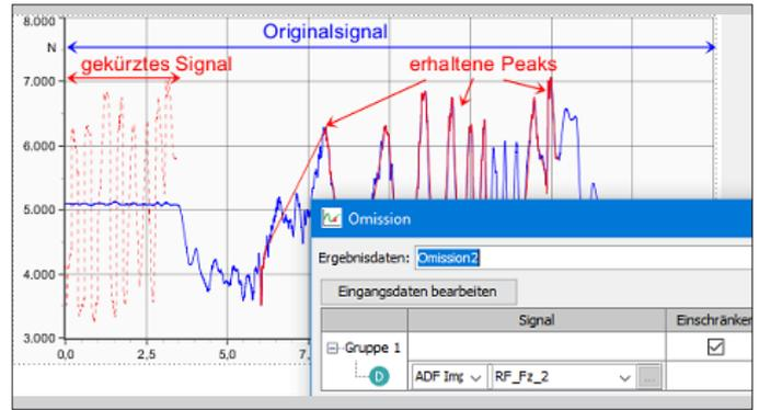
Convenient shortening of any number of measurement signals simultaneously, taking the damage and extremal values into consideration, as preparation for a test run on multi-axial test stands:
