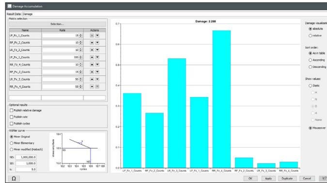
Calculation to evaluate the influence of a load spectrum on the life expectancy of a component. The required input data is provided by the Rainflow analysis.
