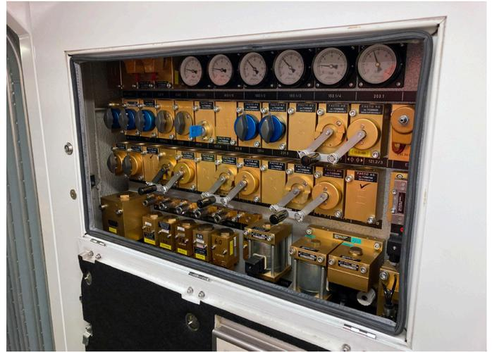
Maintenance is a complex operation: the pneumatic brake system in a local train, with pressure indicators and control valves for all the bogies.
