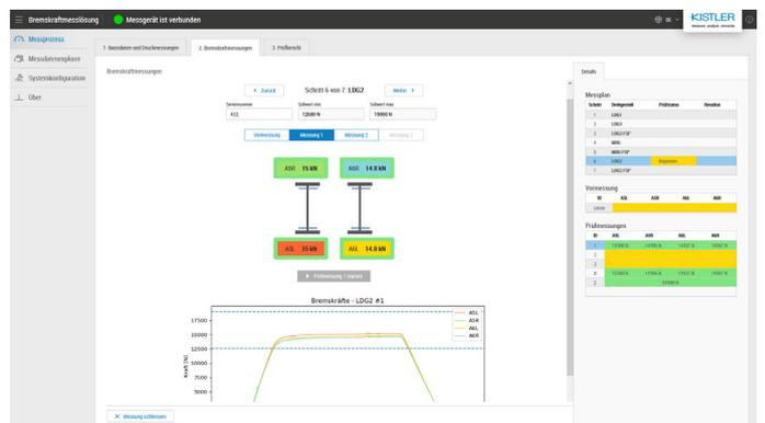
The software for the new Brake Force Measurement Solution (BFMS) developed by Kistler for SBB RICO accurately maps the process steps as well as the brake systems of the trains and the brake forces.
