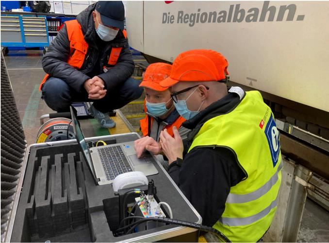
Josua Hunziker, Lead Solutions Architect at Kistler, checks the procedure for brake force measurements.
