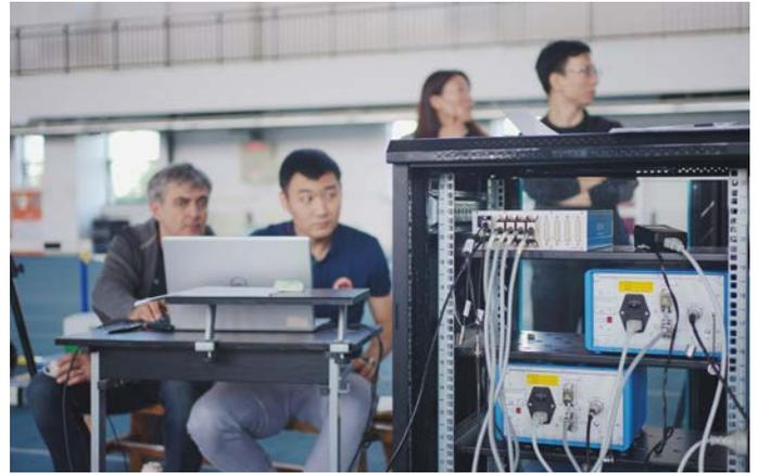
Absolute attention is focused on the vault: the measuring station with evaluation electronics for force plates from Kistler.
