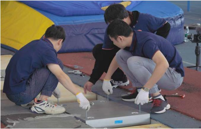
To obtain exact measurements of each pole vaulter's run-up (especially the last three steps), the force plates from Kistler can be repositioned with just a few easy maneuvers.
