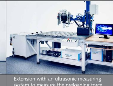
Extension with an ultrasonic measuring system to measure the preloading force
