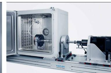
Horizontal ANALYSE system with heat chamber
