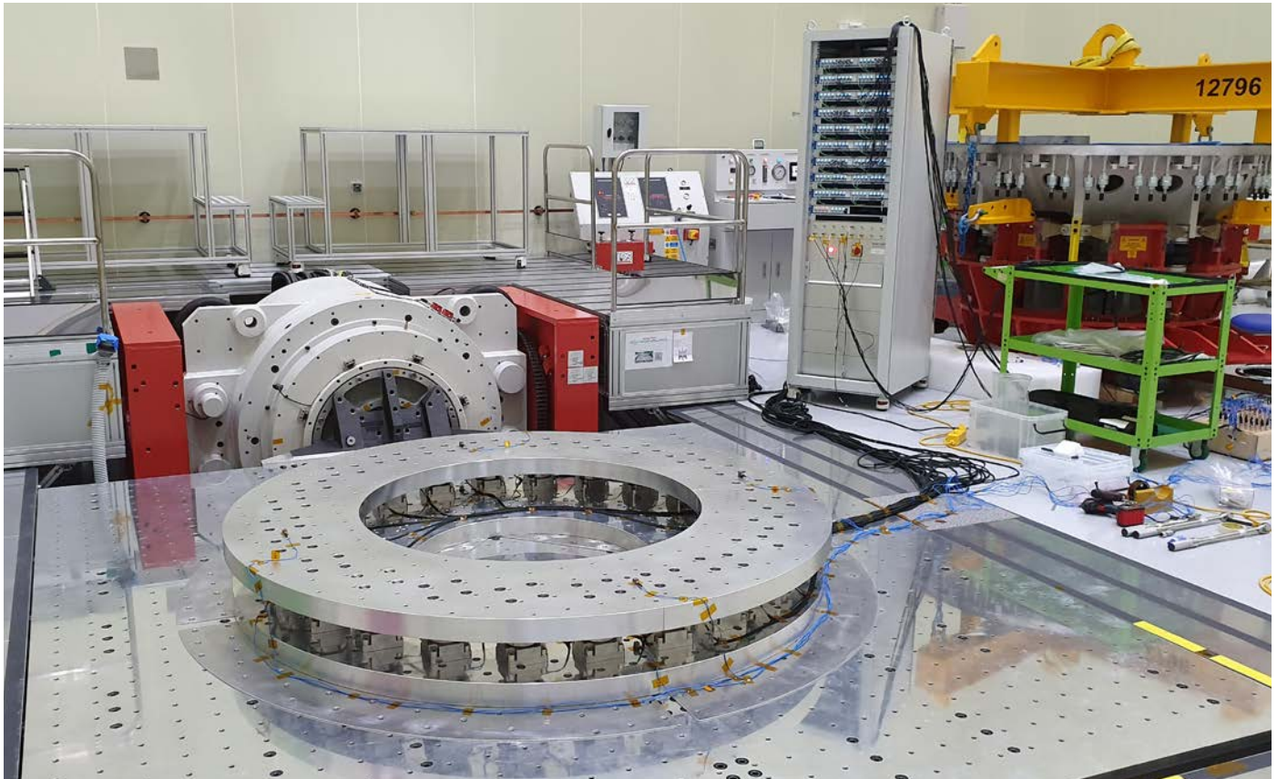
Measurement equipment from Kistler in a ring structure for FLVT.
