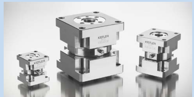
The 9377C force sensor from Kistler is a piezoelectric precalibrated triaxial transducer for forces up to 150 kN.
