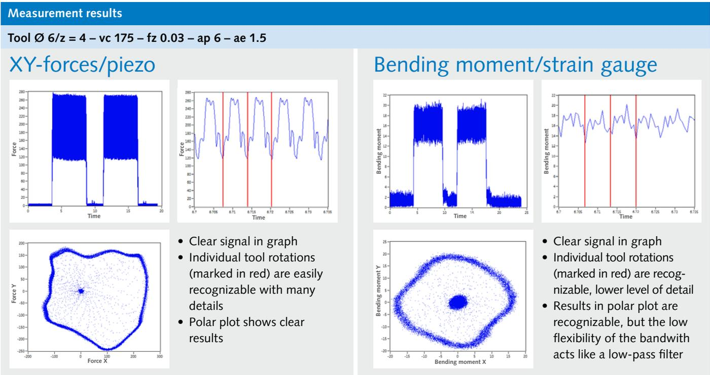
Fig. 5: Comparative values for the action of forces in the x/y directions and bending moment, with a tool diameter of 6 mm
