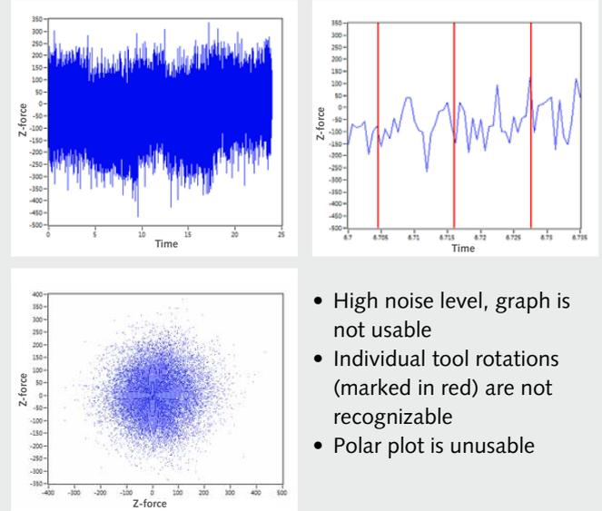
Fig. 7: Comparative values for the action of forces in the z direction with a tool diameter of 6 mm
