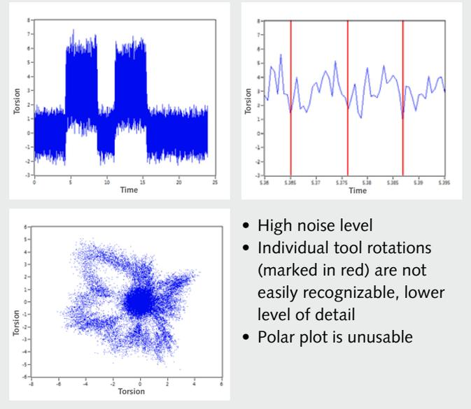
Fig. 3: Comparative values from the torque measurement with a tool diameter of 10 mm
