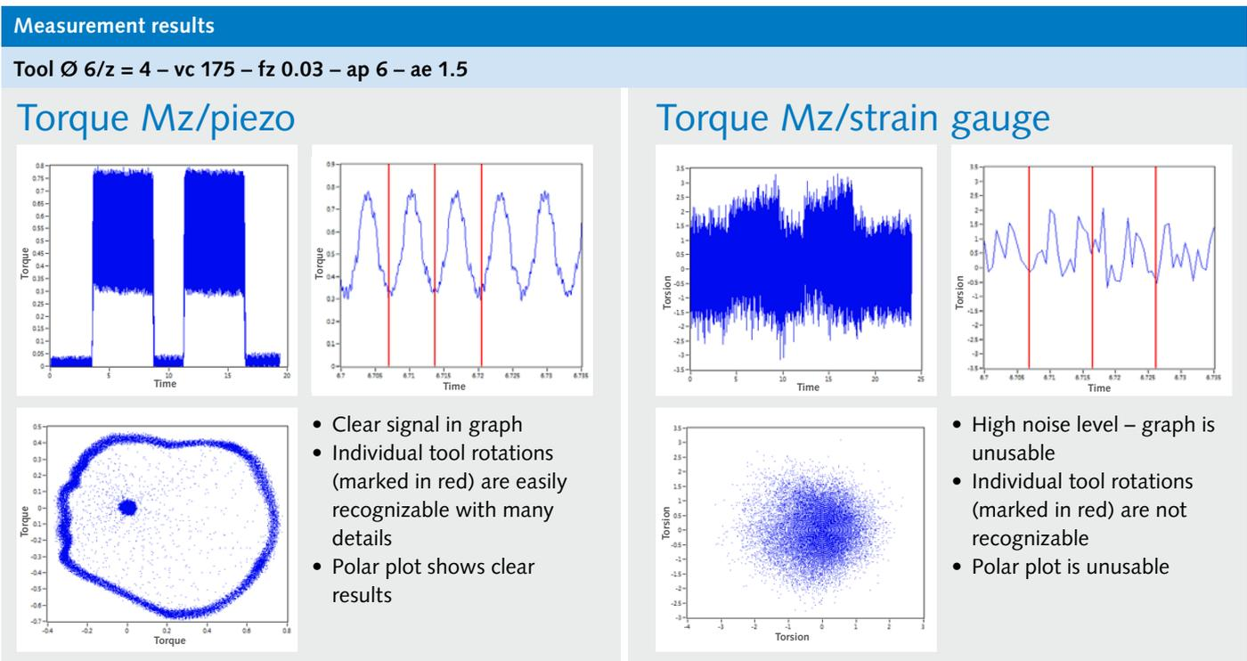
Fig. 6: Comparative values from the torque measurement with a tool diameter of 6 mm
