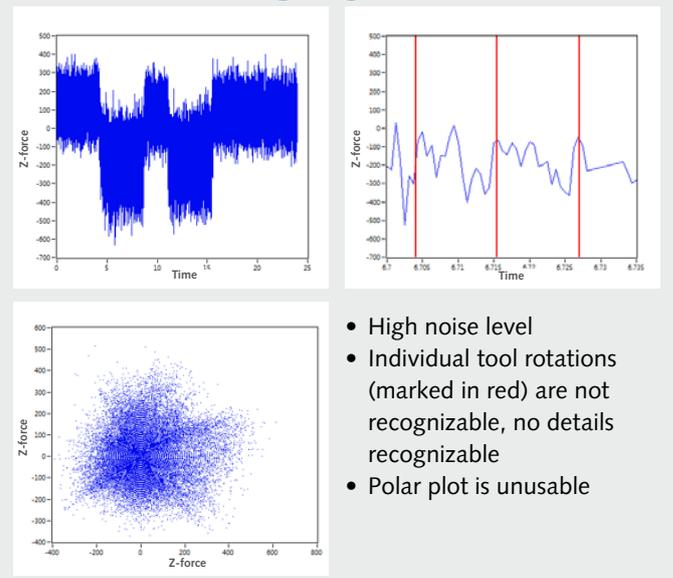
Fig. 4: Comparative values for the action of forces in the z direction with a tool diameter of 10 mm
