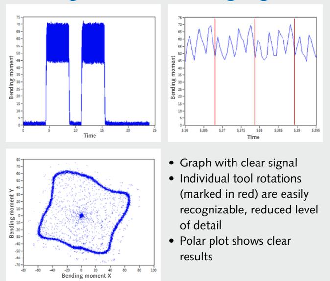
Fig. 2: Comparative values for the action of forces in the x/y directions and bending moment, with a tool diameter of 10 mm
