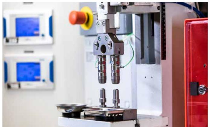
Two 9340A Force Links from Kistler monitor the forces that act during the joining process.
