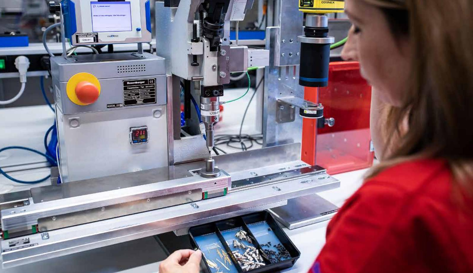
The display of Kistler's maXYmos process monitoring system guides a production employee through the assembly process.
