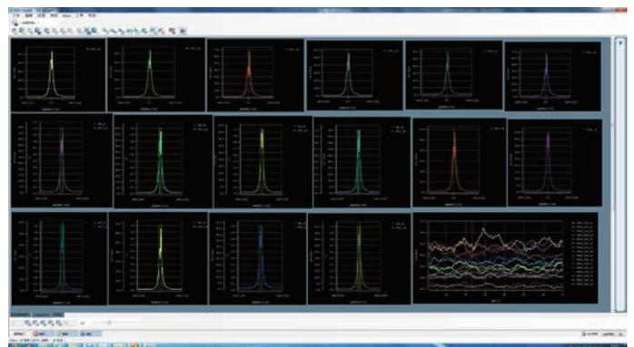
Measurement technology from Kistler allows simultaneous monitoring of injection and internal pressure on all 16 cylinders.
