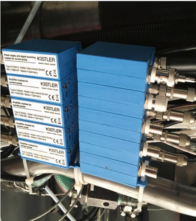
The 2105A current impulse sensor from Kistler helps to optimize injection and ignition timing.
