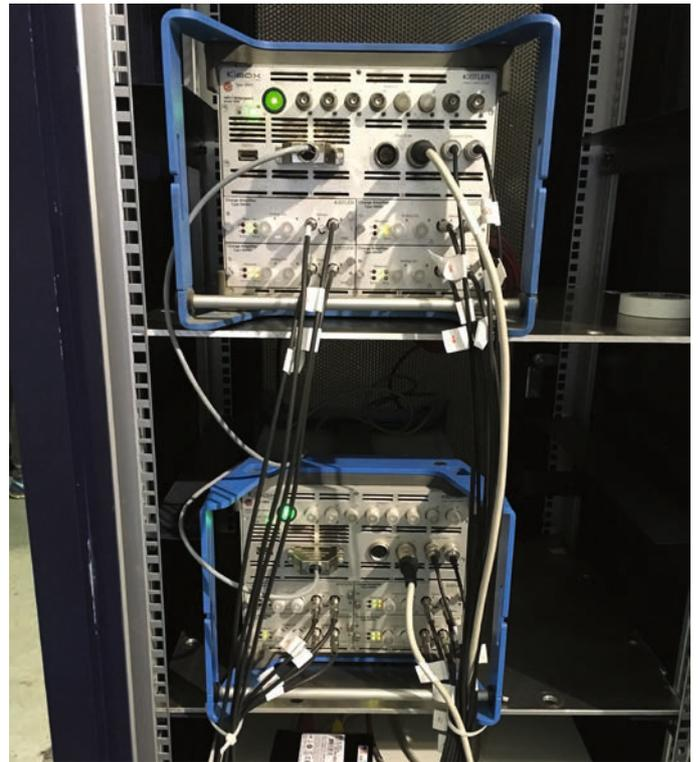
Using two cascading KiBoxes from Kistler, it was possible to monitor and optimize all 16 cylinders simultaneously.
