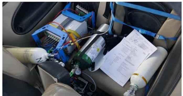
Measuring station in the cockpit; on the left, the KiBox from Kistler for engine indication
