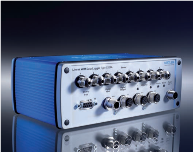
WIM Data Logger: weighing and tire screening in one system
