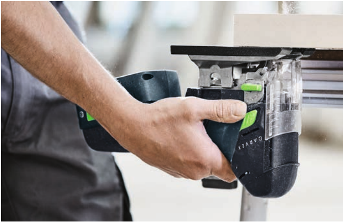
Professionals prefer to saw from below: that gives them optimal visibility of the saw blade and the scribe line.
