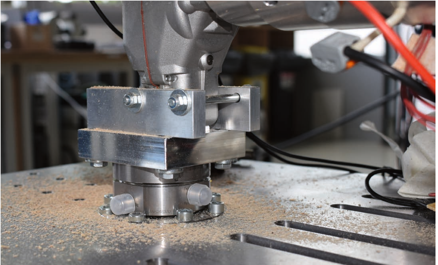
Precise measurements of dynamic forces and moments acting on jigsaws – with the 6-component force/moment sensor from Kistler. The saw is mounted upside-down.
