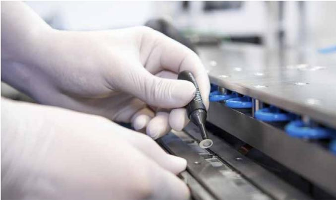
4 Once the quartz crystals are installed, final assembly of the sensor can take place. This includes installing the cables and sealing the sensor to make it airtight and waterproof. Finally, the aluminum profile is enclosed in a foam casing that dampens lateral forces.
